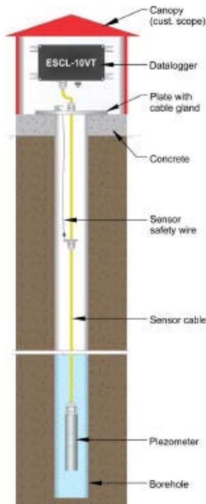
Typical installation scheme for automatic groundwater monitoring system
