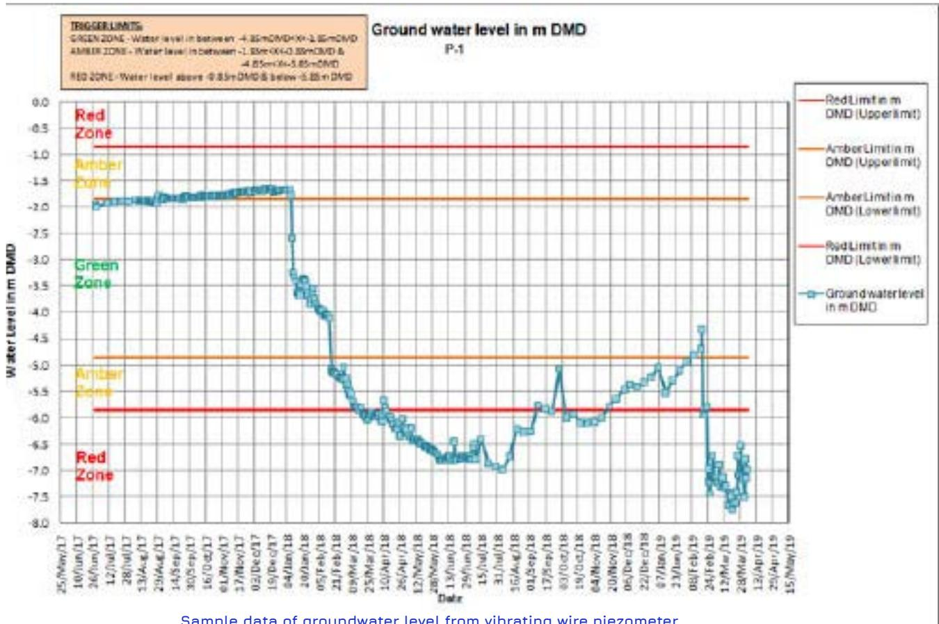
Sample data of groundwater level from vibrating wire piezometer
