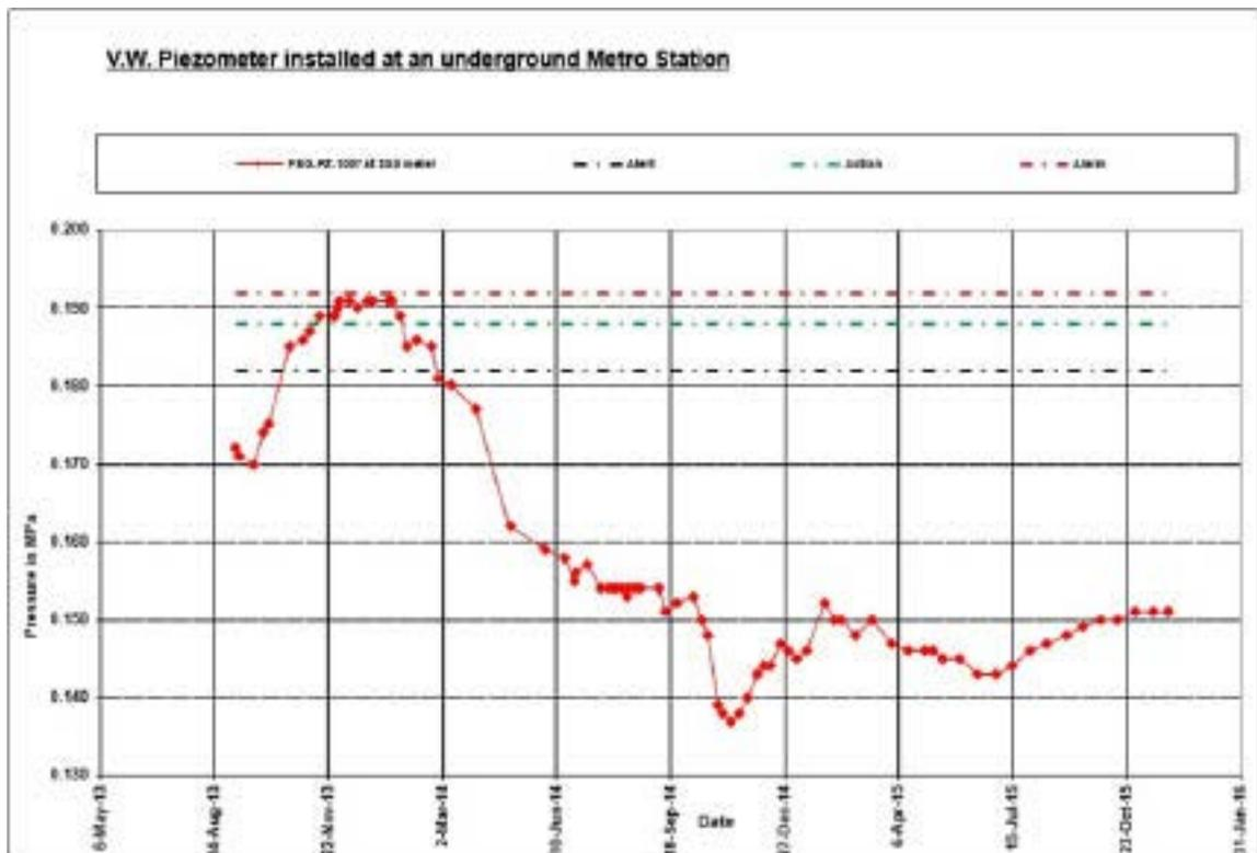
Sample data from vibrating wire piezometer
