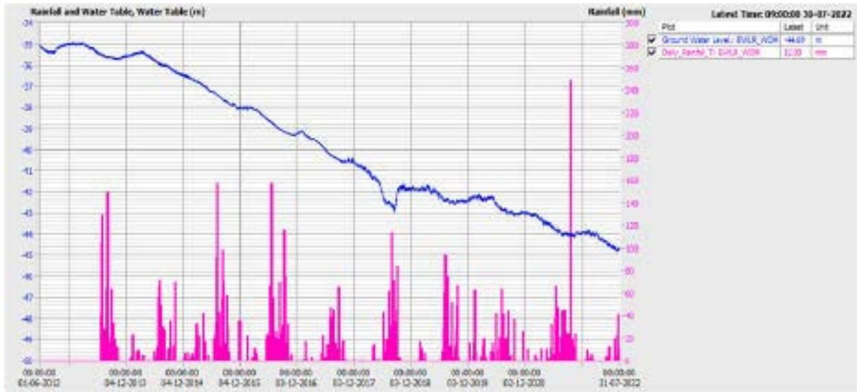
Online groundwater level and rainfall data from a factory in Lucknow. It is observed that water level increases a little after each monsoon. Yet it has recorded long-term water level decline with almost same amount of rainfall, due to extensive groundwater use.
